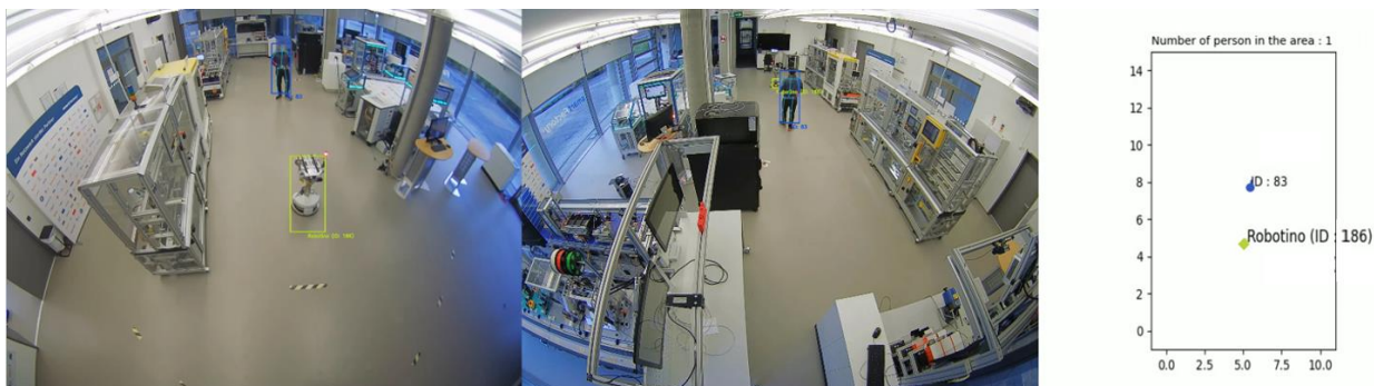
Figure 21: Example of human and object detection, 3D geolocalisation, tracking (done separately for objects and humans) and robot's identification with merge from 2 cameras in which the robot is moving.
