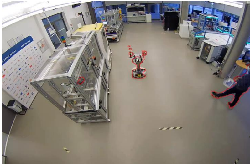
Figure 19: Background subtraction - moving object detection based on Gaussian model. Some false alarms - shiny reflections in left workstation
