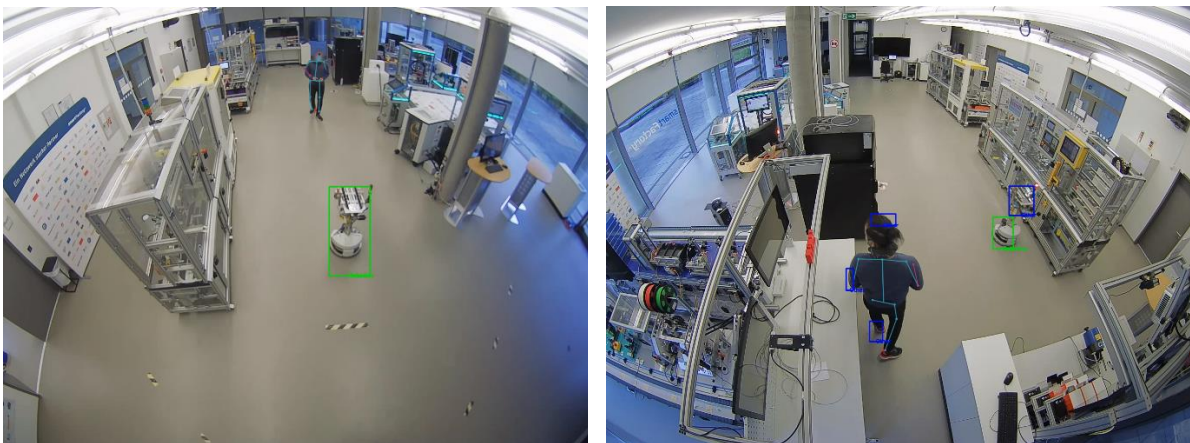
Figure 7: Result of Robotino identification (green) using Resnet features and One-Class SVM applied to background subtraction’s detected moving objects (bounding boxes)
