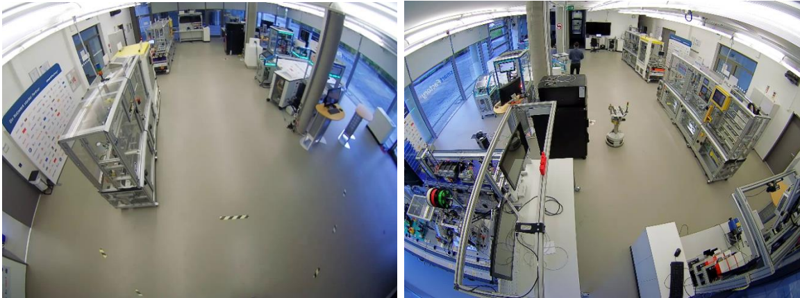
Figure 15: DFKI platform – 3 workstations, robots and 2 cameras
