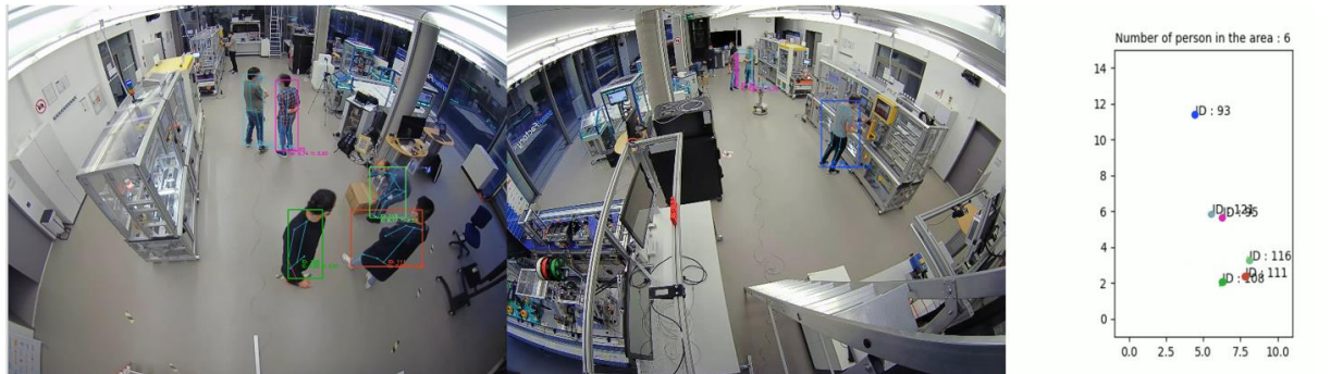
Figure 20: Example of human detection, 3D geolocalisation and tracking with merge from 2 cameras.
