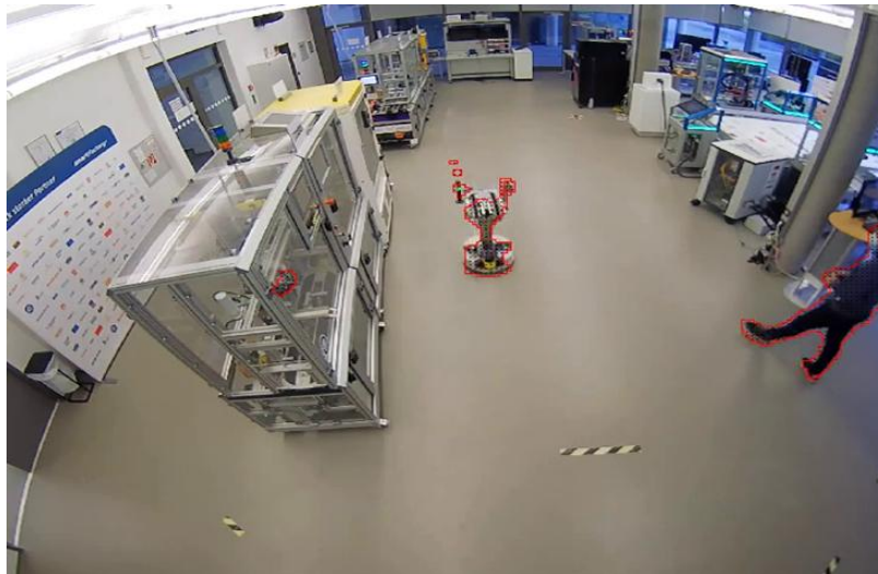
Figure 17 : Background subtraction - moving object detection based on Gaussian model. Some false alarms - shiny reflections in left workstation
