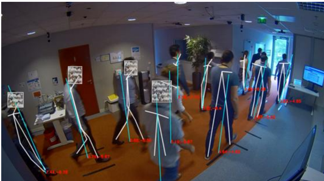
Figure 10 : Skeleton detection and 3D location with key points (feet, hip, shoulder) projection
