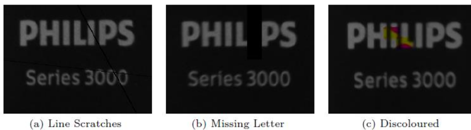
Figure 5. Artificially generated defect classes (open-set) used for testing.
