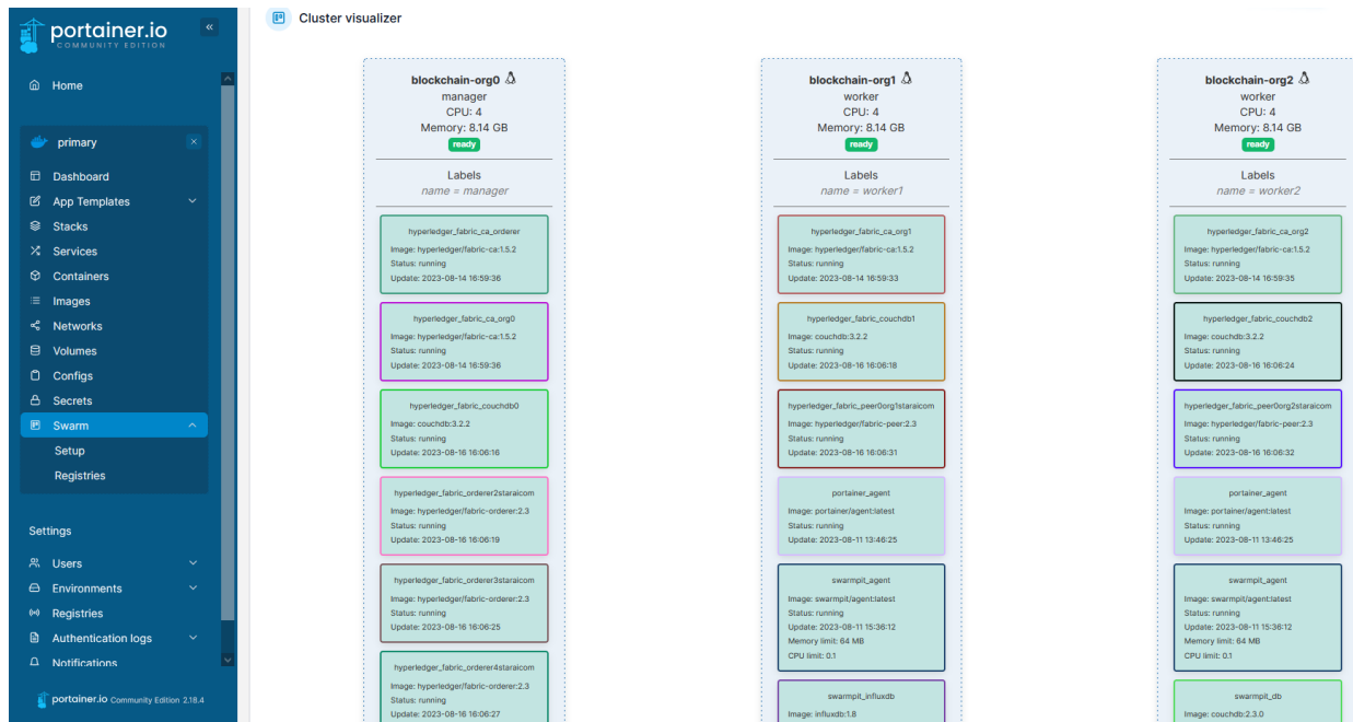
Figure 49: The distribution of running services among nodes as visualised in Portainer
