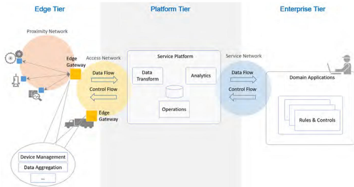
Figure 3: Outline of a Three Tier Architecture for IIoT systems in-line with the IIRA
